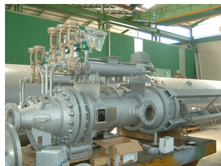
Mounting and testing of filter in workshop. Final packing of filters for shipment
